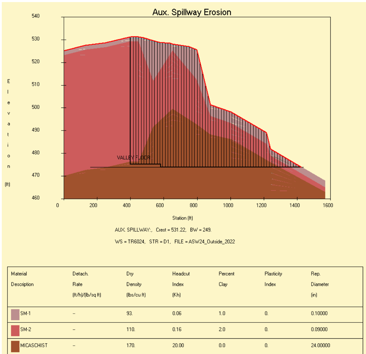
Figure 3-6. Plot of auxiliary spillway outside edge profile and extent of erosion from integrity analysis for existing conditions 24-hour PMF obtained from SITES model output.
