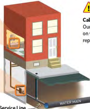
Water Service Line May be made of lead, copper, galvanized steel or plastic.
