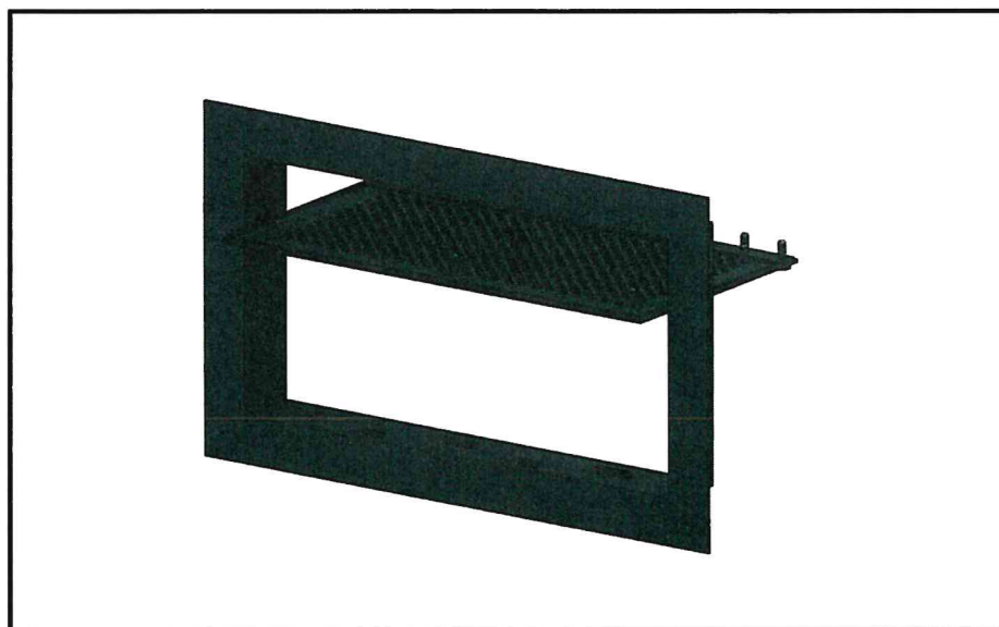
FIGURE 2—MODEL FFV-1608 FREEDOM FLOOD VENT™: SHOWN WITH FLOOD DOOR PIVOTED OPEN
